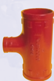
Figura 55 TE reductora Gama 2 1/2"x2" - 8"x6" (65x50-200x150 mm)
