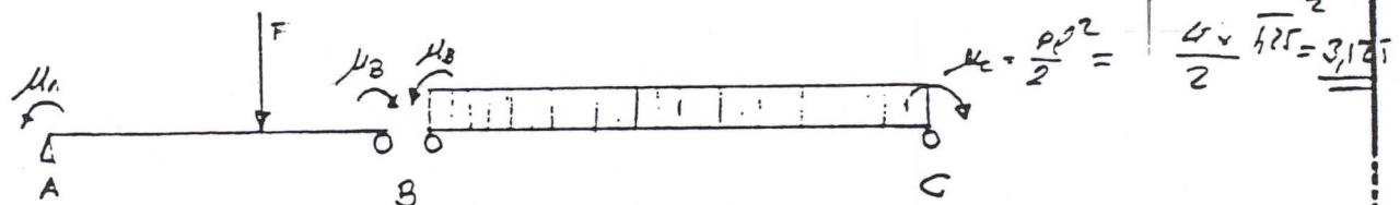
$$\frac{\mu_B}{\mu} = \frac{\mu_B (2\ell)}{3EI} \quad \frac{\psi_B}{\mu} = \frac{\mu_B (2\ell)}{6EI} \quad \frac{\psi_{BD}}{\mu} = \frac{\mu_B (3\ell)}{6E(3I)} \quad \frac{\psi_C}{\mu} = \frac{\mu_C (3\ell)}{3E(3I)}$$
